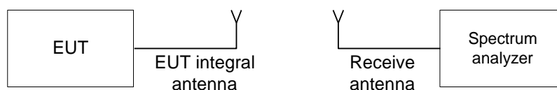
Figure 7.1.1 Setup for transmitter shut down test
