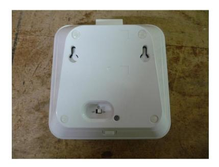
Photograph No.3 ES7502HC Care Home Control panel rear side view with backplane removed
