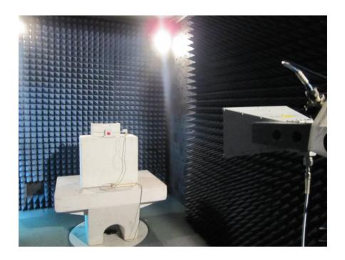
${\bf Photograph~No.4}\\ {\bf Setup~for~field~strength~emission~measurements~at~the~OATS~in~30-200~MHz~range}$
