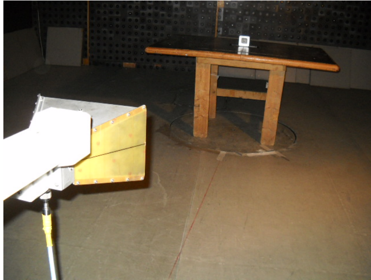
Photograph 8.1.2 Setup for radiated emission measurements, general view
