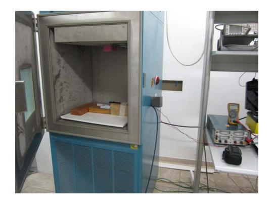
Photograph No.10 Setup for frequency stability measurements
