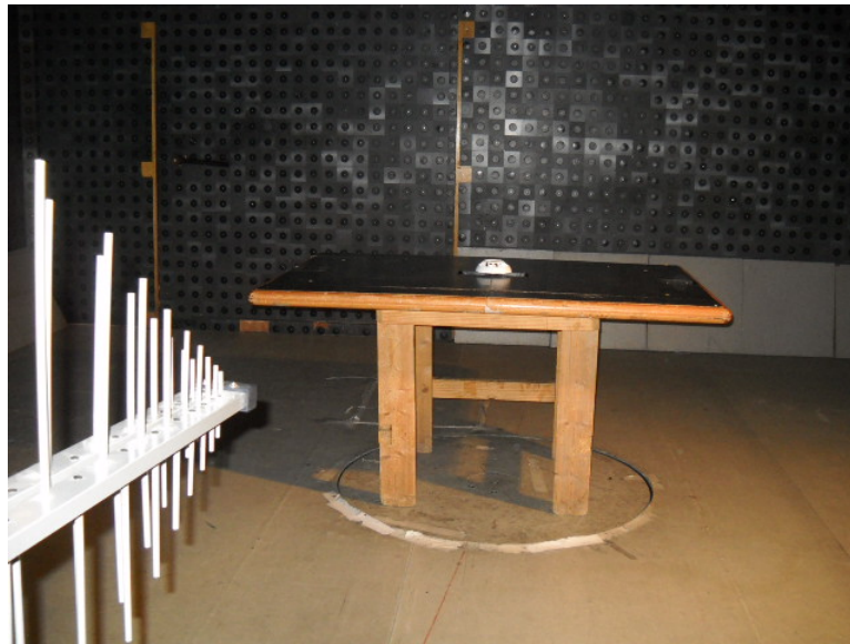
Photograph 8.1.1 Setup for final radiated emission measurements
