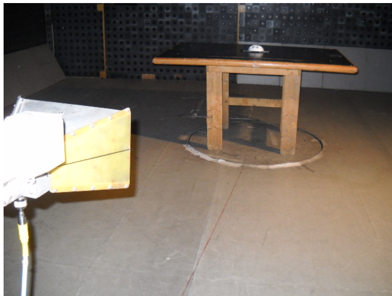
Photograph 8.1.2 Setup for final radiated emission measurements
