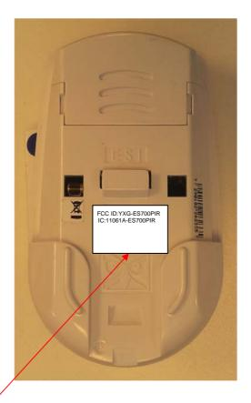
Label with FCC ID:YXG-ÉS700PIR and IC:11061A-ES700PIR is located at the rear side panel. The statement according to FCC part 15 §15.19(a)(3) is placed in User's Guide (Application exhibit User\_manual\_24393, page 2).
