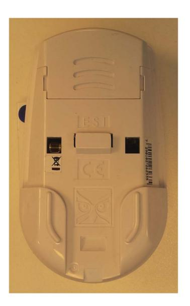
Photograph No.3 ES700PIR passive infrared detector rear side view
