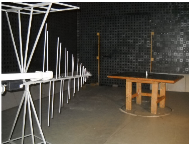
Photograph 8.1.1 Setup for radiated emission measurements
