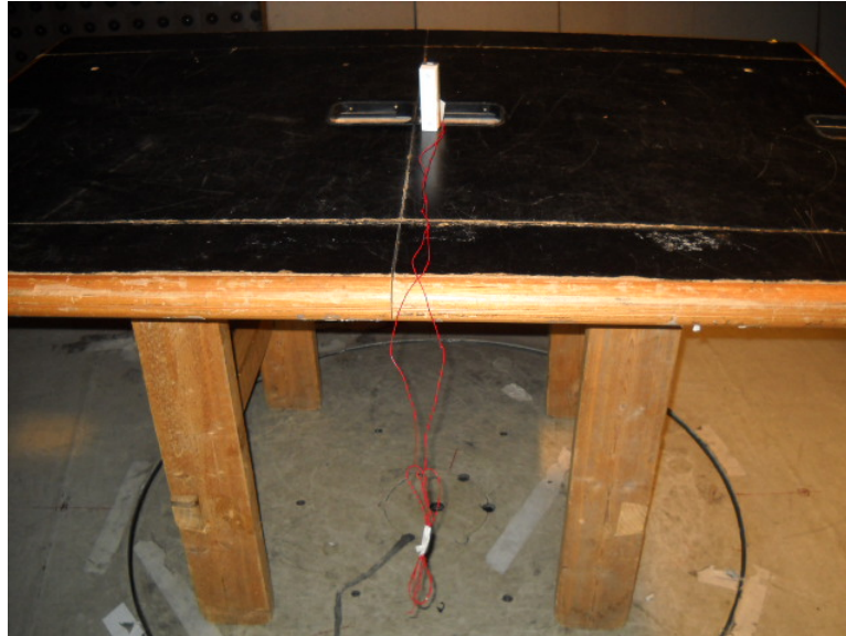
Photograph 8.1.2 Setup for radiated emission measurements, EUT close view
