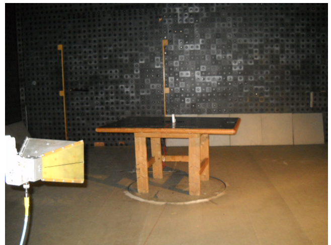
Photograph 8.1.1 Setup for radiated emission measurements
