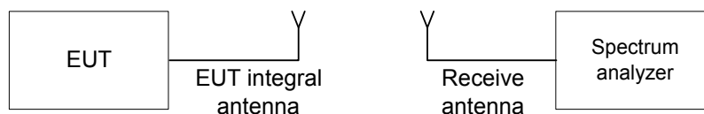
Figure 7.1.1 Setup for transmitter shut down test
