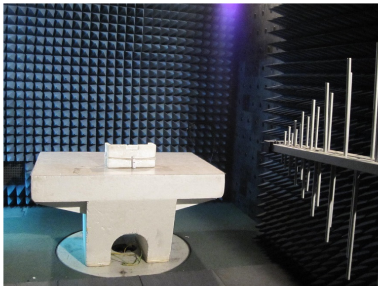
Photograph 8.1.1 Setup for radiated emission measurements
