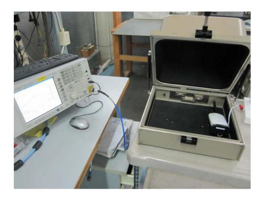
Photograph No.8 Setup for occupied bandwidth measurements
