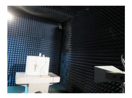
${\bf Photograph~No.4}\\ {\bf Setup~for~field~strength~emission~measurements~at~the~OATS~in~30-200~MHz~range}$
