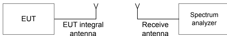
Figure 7.1.1 Setup for transmitter shut down test
