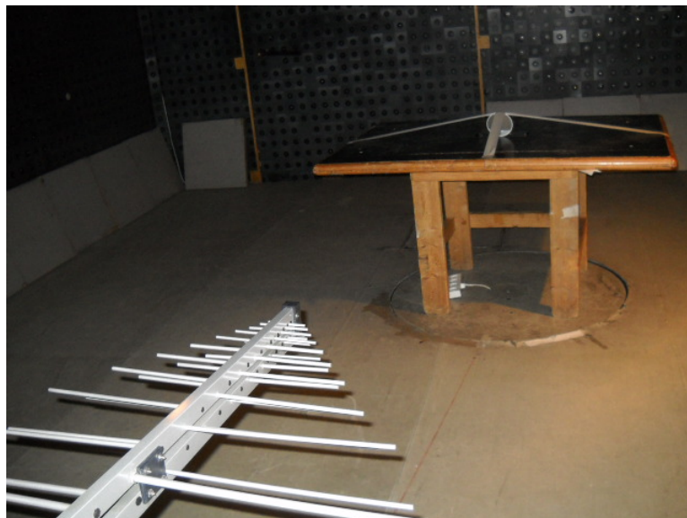
Photograph 8.1.1 Setup for radiated emission measurements
