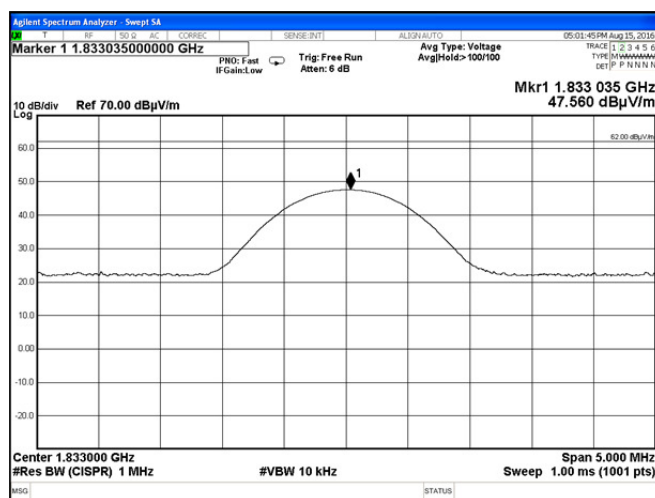
Plot 7.2.8 Radiated emission measurements at the second harmonic frequency
