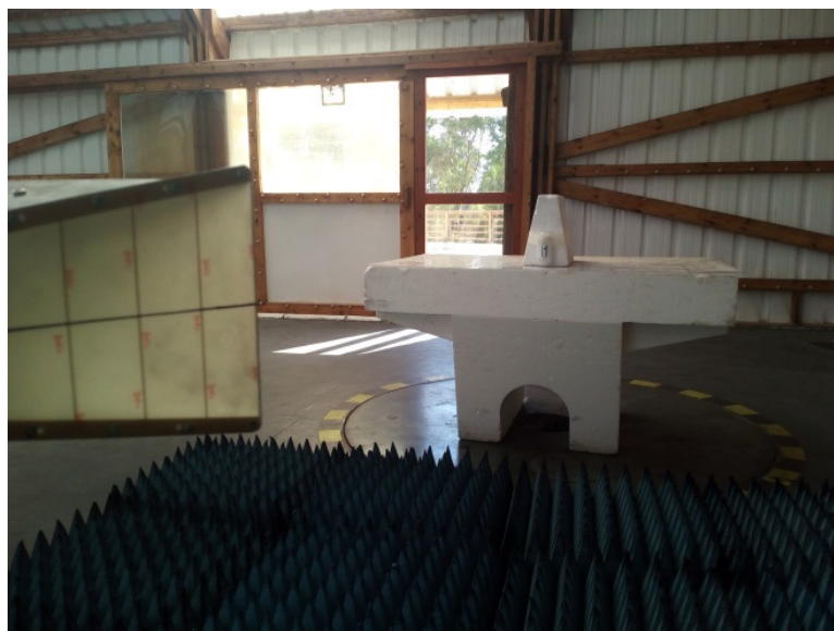
Photograph 8.1.4 Setup for radiated emission measurements at the OATS, general view
