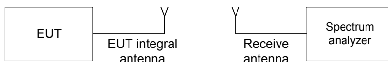
Figure 7.1.1 Setup for transmitter shut down test
