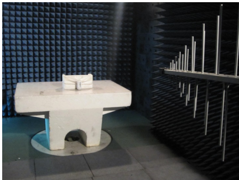
Photograph 8.1.1 Setup for radiated emission measurements in the anechoic chamber
