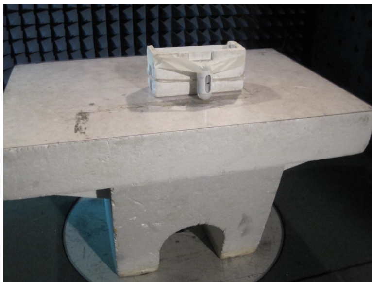
Photograph 8.1.3 Setup for radiated emission measurements in the anechoic chamber, EUT close view
