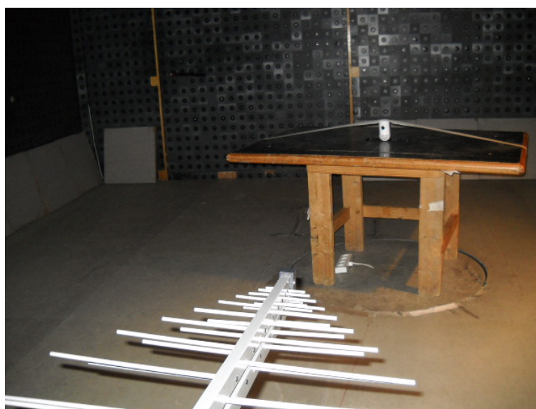
Photograph 8.1.1 Setup for radiated emission measurements
