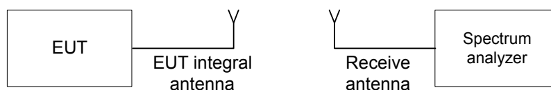
Figure 7.1.1 Setup for transmitter shut down test
