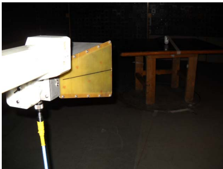
Photograph 8.1.2 Setup for final radiated emission measurements
