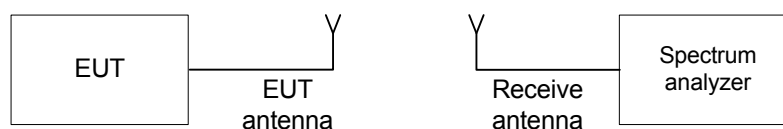
Figure 7.3.1 Occupied bandwidth test setup
