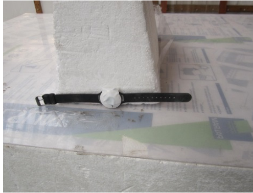
Photograph 6.4.2 EUT with strap in Y-axis orthogonal position
