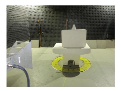
${\bf Photograph~No.4}\\ {\bf Setup~for~carrier~emission~measurements~at~the~OATS~in~30-1000~MHz~range}$
