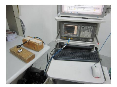
Photograph No.6 Setup for occupied bandwidth measurements
