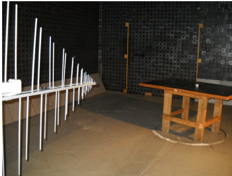
Photograph 8.1.1 Setup for radiated emission measurements
