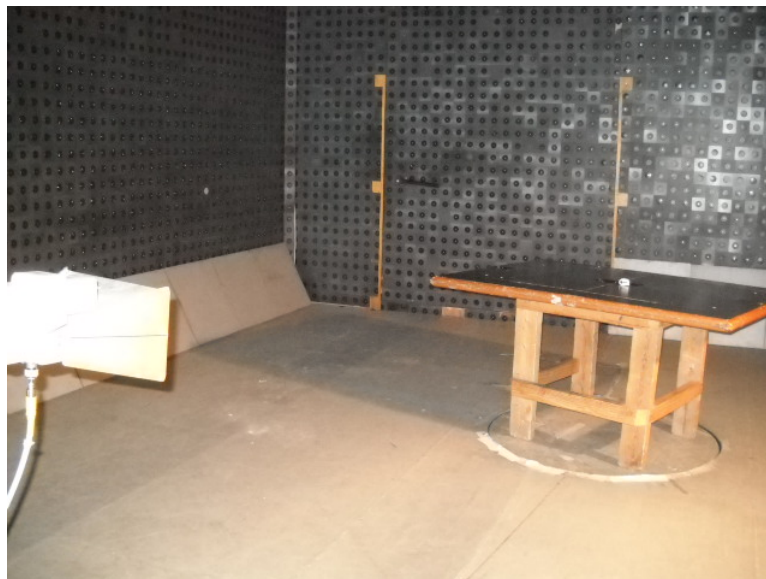
Photograph 8.1.2 Setup for radiated emission measurements
