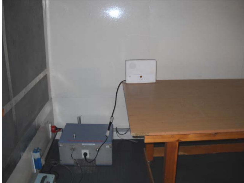
Photograph No.4 Setup for conducted emission measurements on AC power lines
