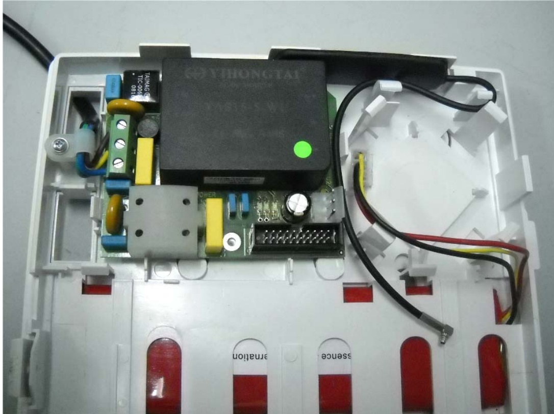
Photograph No.3 ES7000EG wireless control panel internal view with main PCB removed
