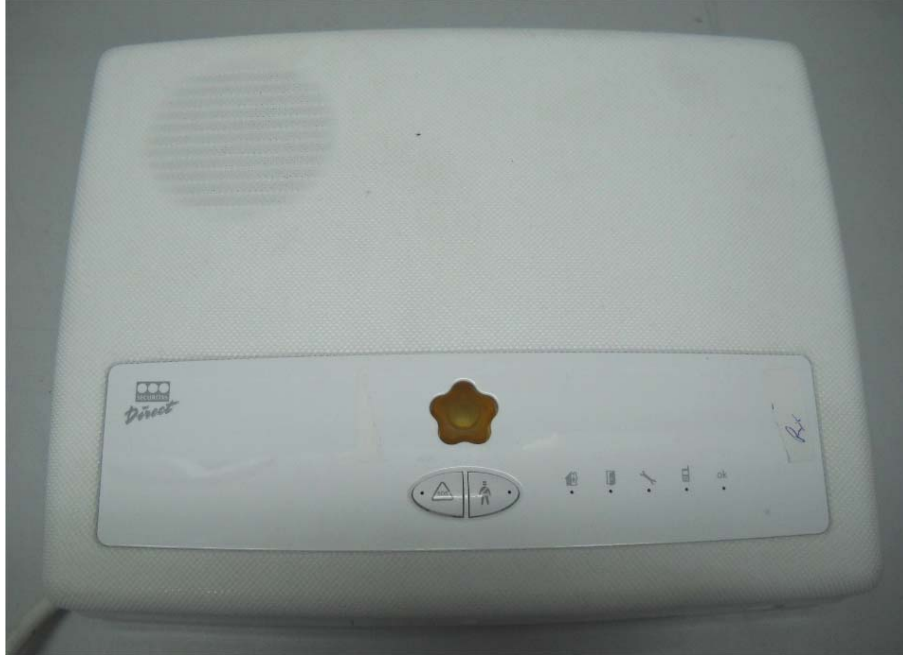
Photograph No.1 ES7000EG wireless control panel front view
