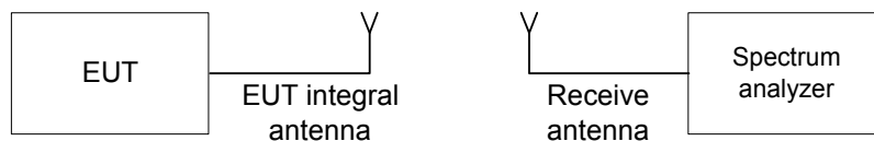
Figure 7.1.1 Setup for transmitter shut down test
