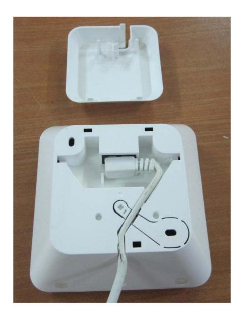
Photograph No.4 ES6502VSF control panel rear side with cover removed
