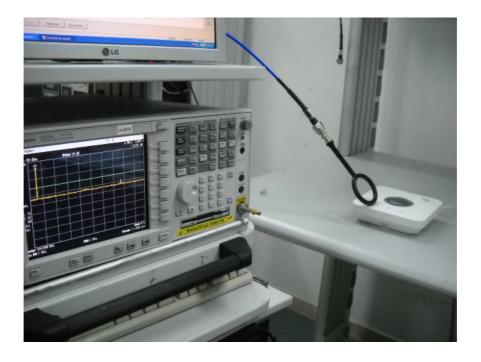
Photograph No.4 Setup for periodic operation measurements
