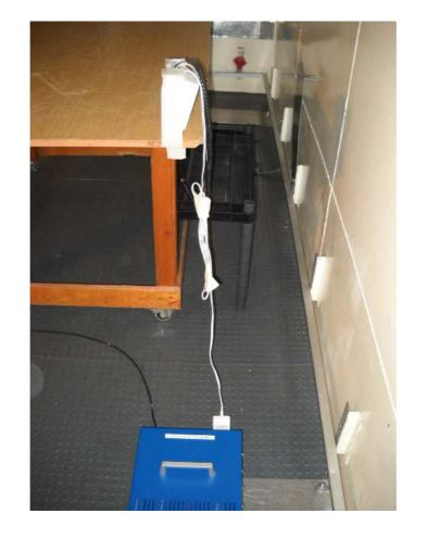
Photograph No.6 Setup for conducted emission measurements on AC power lines
