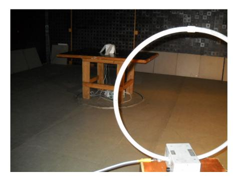
Photograph No.2 Setup for carrier, spurious emission field strength and OBW measurements in the anechoic chamber in 30 – 1000 MHz range
