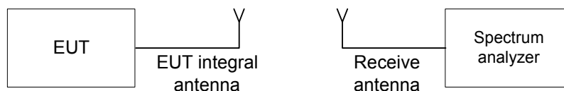
Figure 7.1.1 Setup for transmitter shut down test
