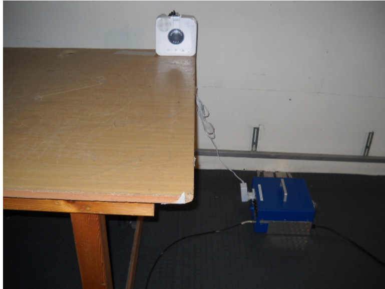
Photograph 8.1.1 Setup for conducted emission measurements
