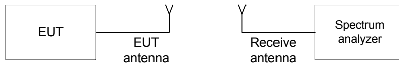
Figure 7.2.1 Occupied bandwidth test setup
