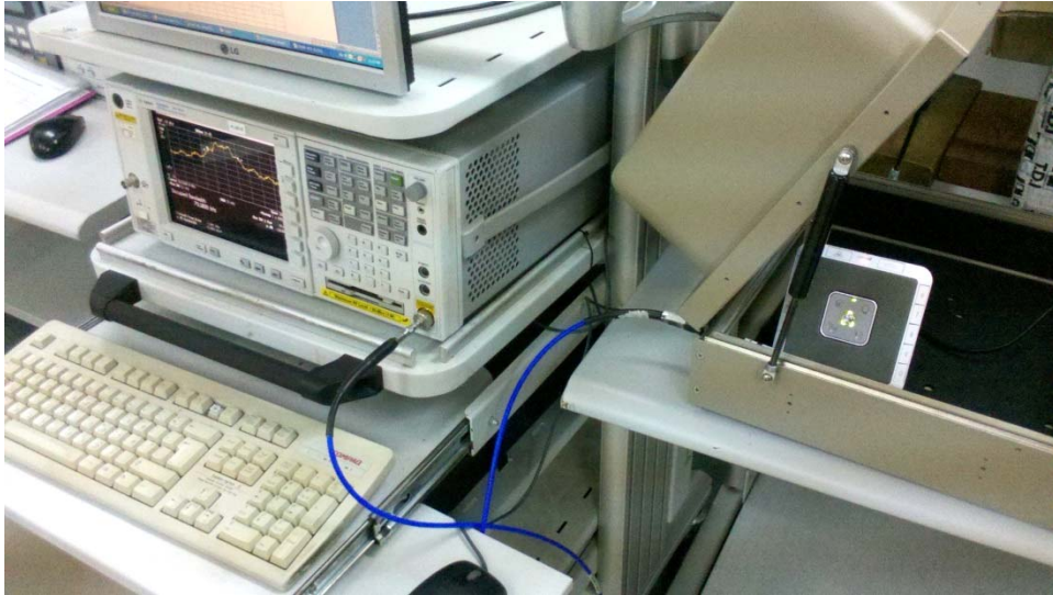
Photograph No.6 Setup for occupied bandwidth measurements
