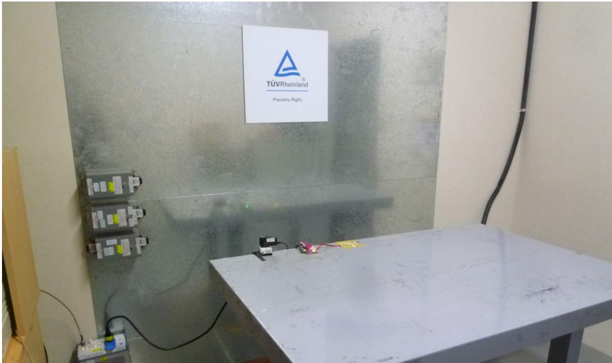
Photograph 9: Set-up for Mains Conducted testing Front
