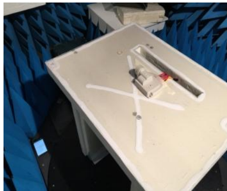
Test setup in anechoic chamber, axis XY
