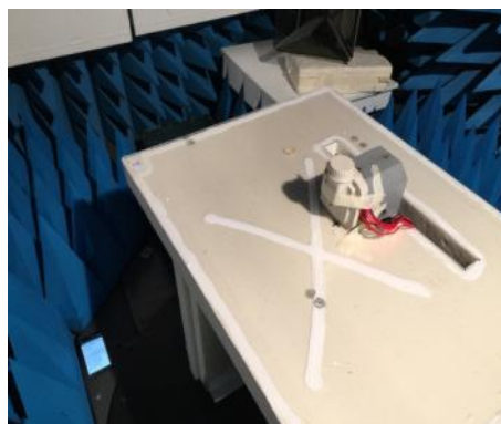
Test setup in anechoic chamber, axis Z
