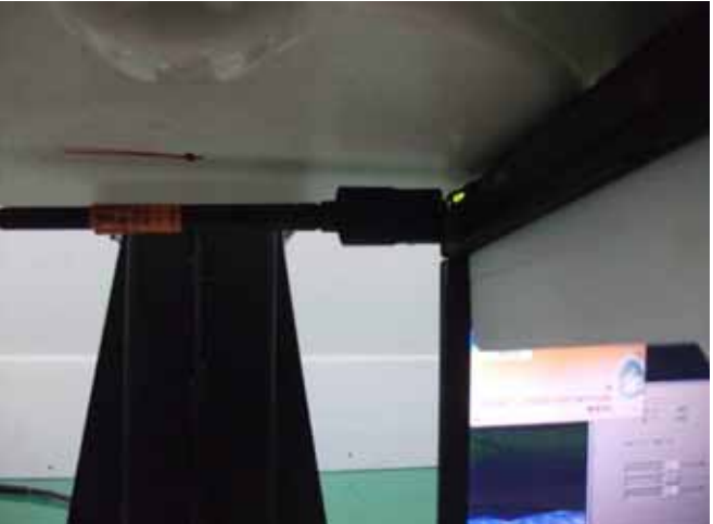
Right side with 180 degree antenna(5mm gap)
