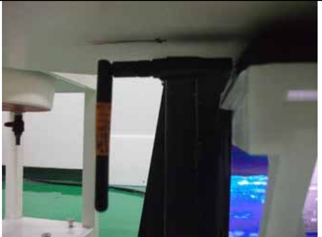
Back side with 90 degree antenna(5mm gap)
