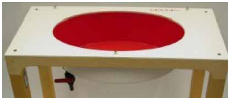
Figure 6 SAM Twin phantom and ELI phantom
