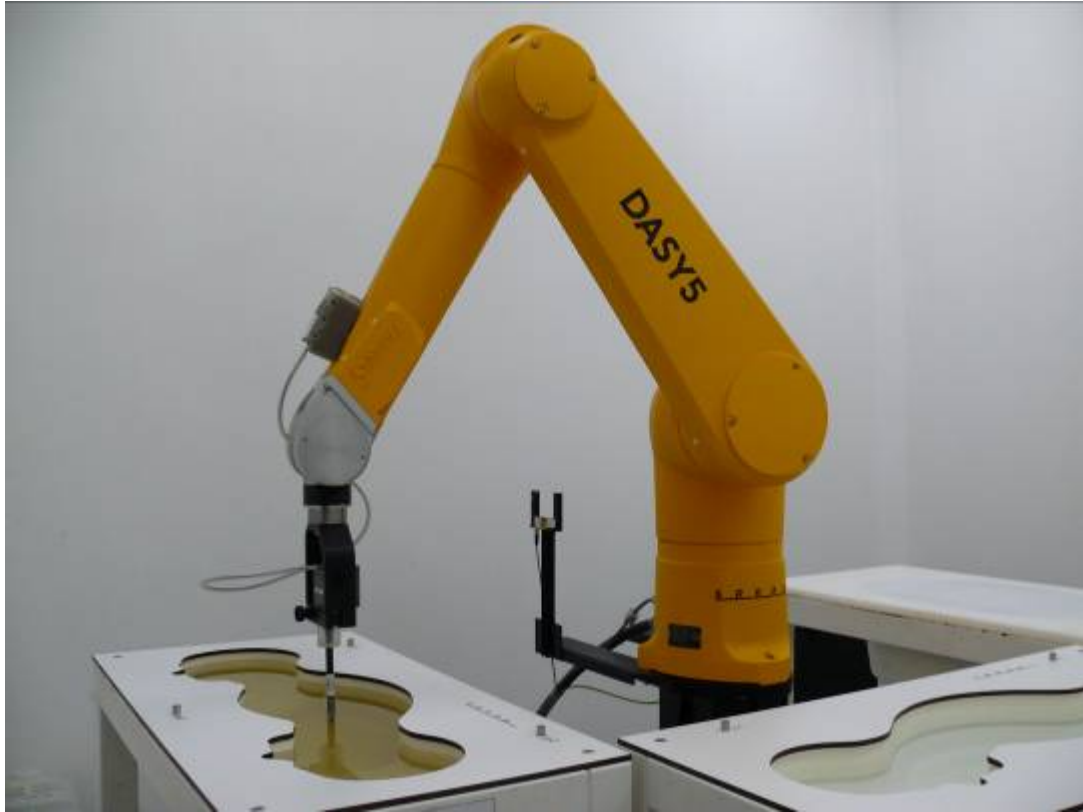
Picture 2: Specific Absorption Rate Test Layout
