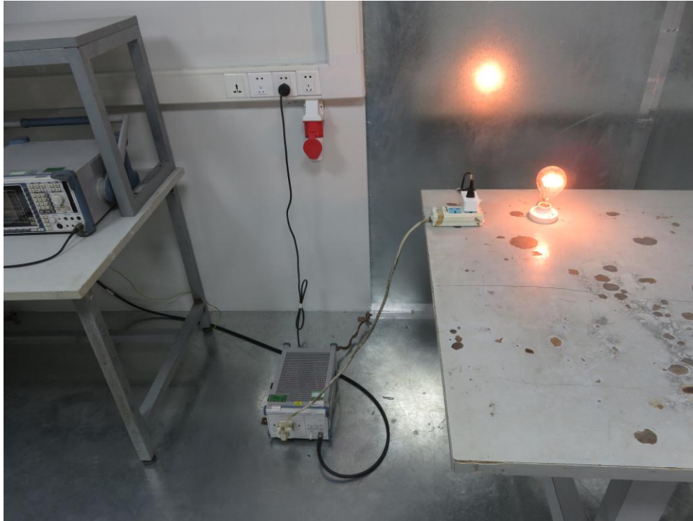
Photo of Conducted Emission Measurement
