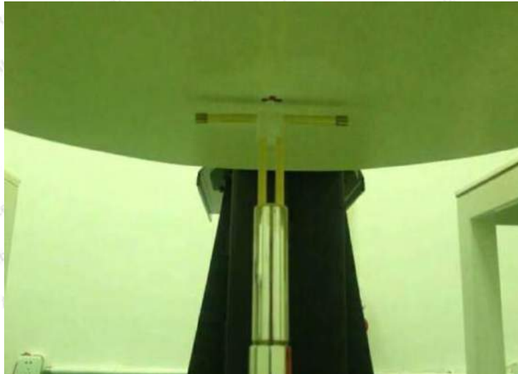
Photo of Dipole Setup
