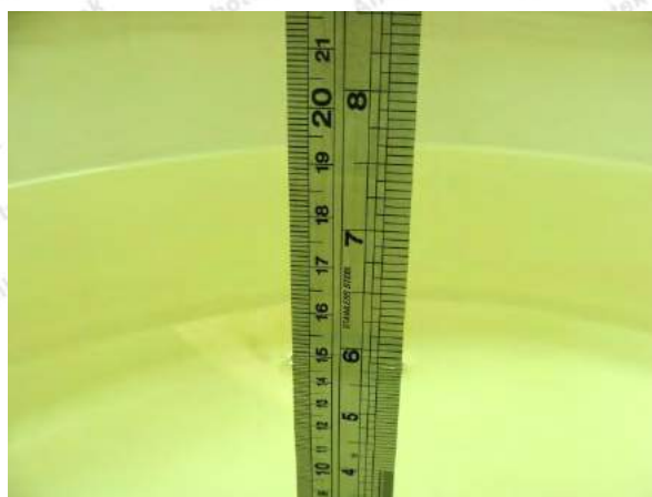
Photo of Liquid Height for Body SAR
