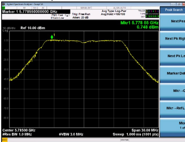
(802.11a) PSD plot on channel 157
