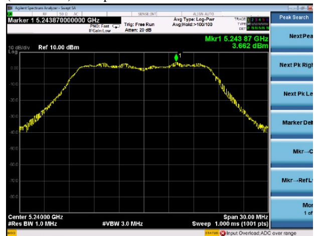
(802.11n20) PSD plot on channel 48
