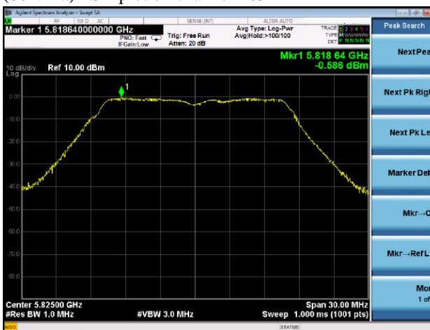
(802.11a) PSD plot on channel 165
