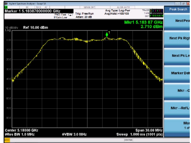
(802.11n20) PSD plot on channel 36
