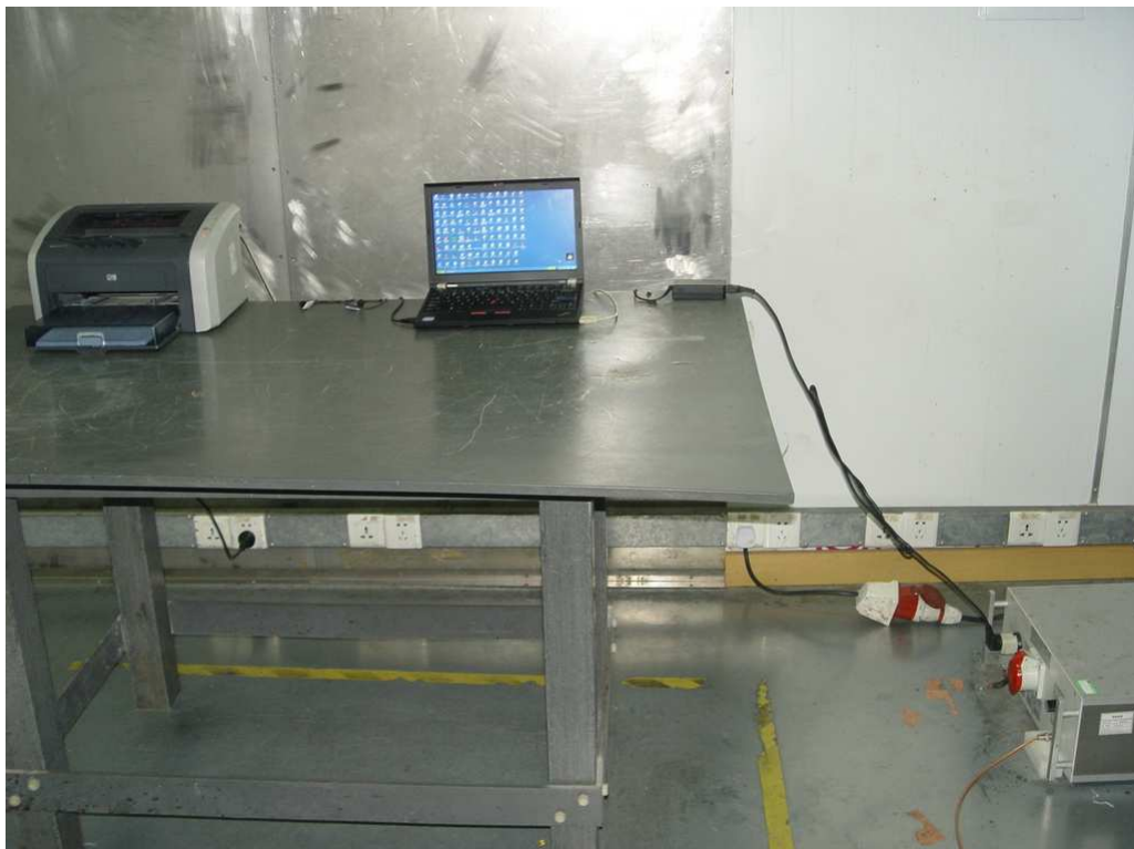
Photograph 6: Set-up for Conducted emissions
