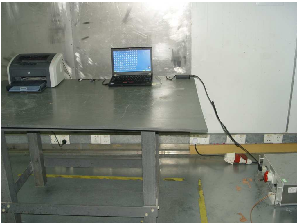
Photograph 6: Set-up for Conducted emissions
