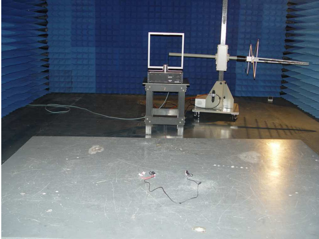
Photograph 2: Set-up for Spurious Emissions (30MHz-1GHz)
