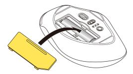
Replacing the battery...
