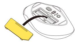
Replacing the battery...
