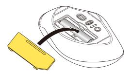
Replacing the battery...
