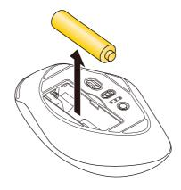
3) Insert the battery according to the positive (+) and negative (-) marks indicated in the battery compartment.
