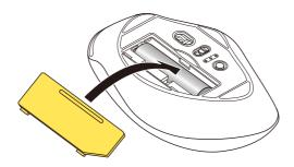
Replacing the battery...
