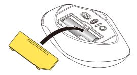
Replacing the battery...
