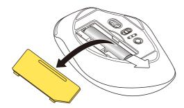
2) Remove the battery insulating tab.
