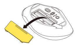
2) Remove the battery insulating tab.
