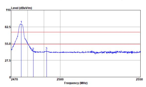
Test Mode: 01; Polarity: Vertical; Modulation:GFSK; Channel:High
