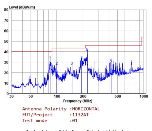
Test Mode: 01; Polarity: Horizontal
