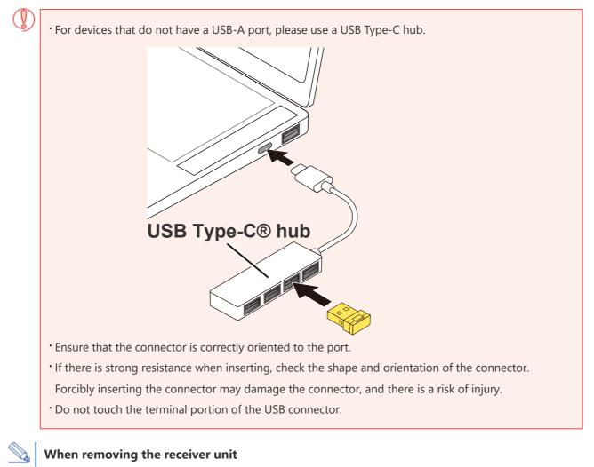
This product supports hot plugging. The receiver unit can be removed while the PC is on.
