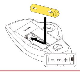
Ensure that the battery is inserted with the positive (+) and negative (-) terminals oriented correctly.
