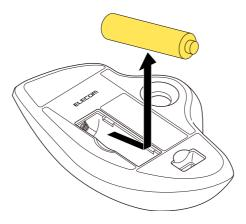
3) Insert the battery according to the instructions on the battery compartment.
