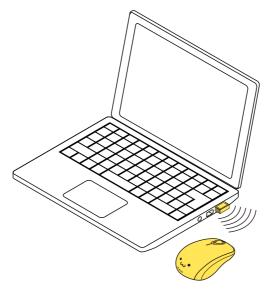
• Connect the Bluetooth receiver to a USB2.0 hub or to an extension cable.
