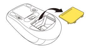
2) Insert the battery at an angle with the battery removal sheet underneath.
