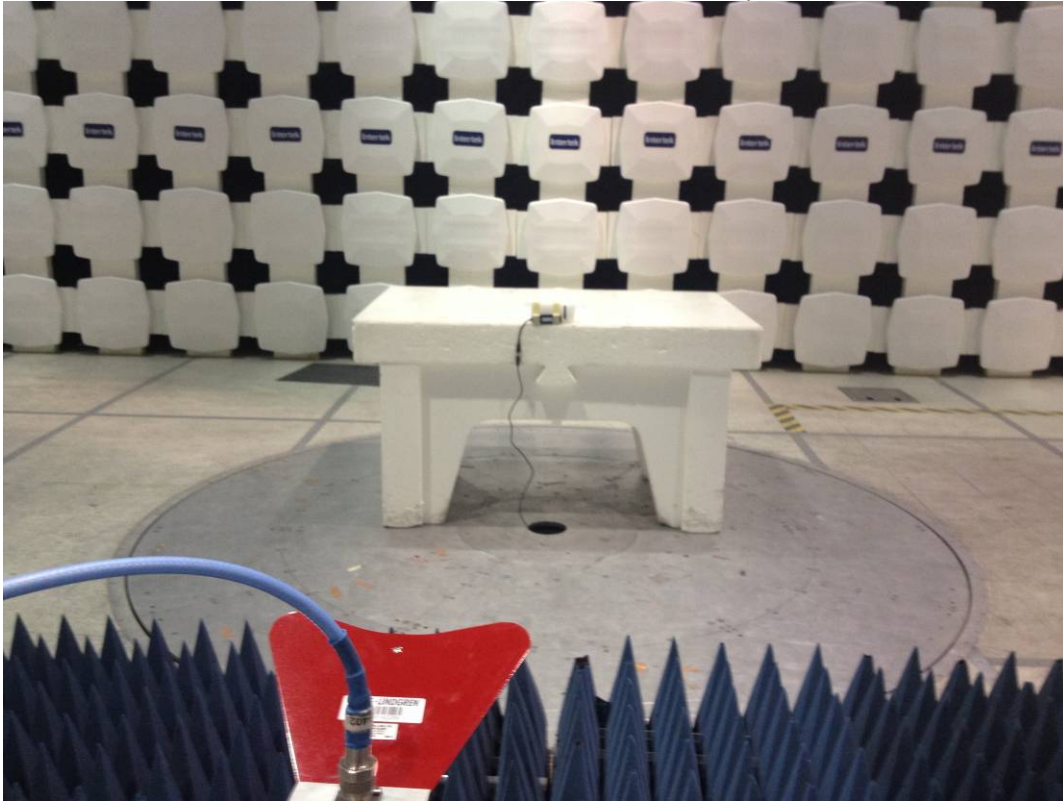
Y axis Radiated Emissions Test Setup
