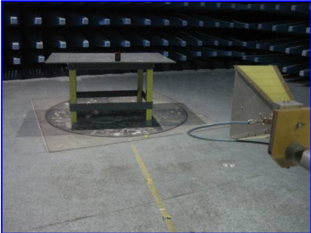
Front View of Radiated Emission Test Setup above 1GHz
