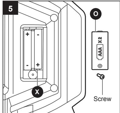
**NOTE:** When changing the clock batteries, all settings will be erased. To avoid this, attach the battery pack or plug in the power adaptor, and turn the unit ON before replacing the clock batteries.
