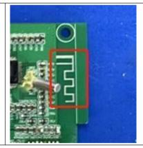
The antenna is PCB antenna. The best case gain of the antenna is 0 dBi.
