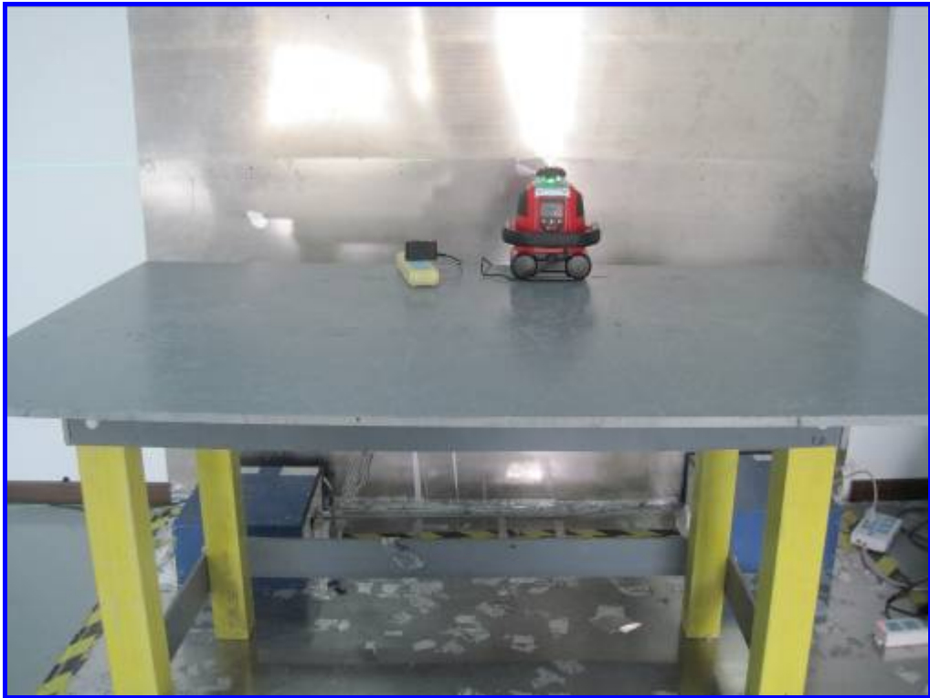
Front View of Conduced Emission Test Setup
