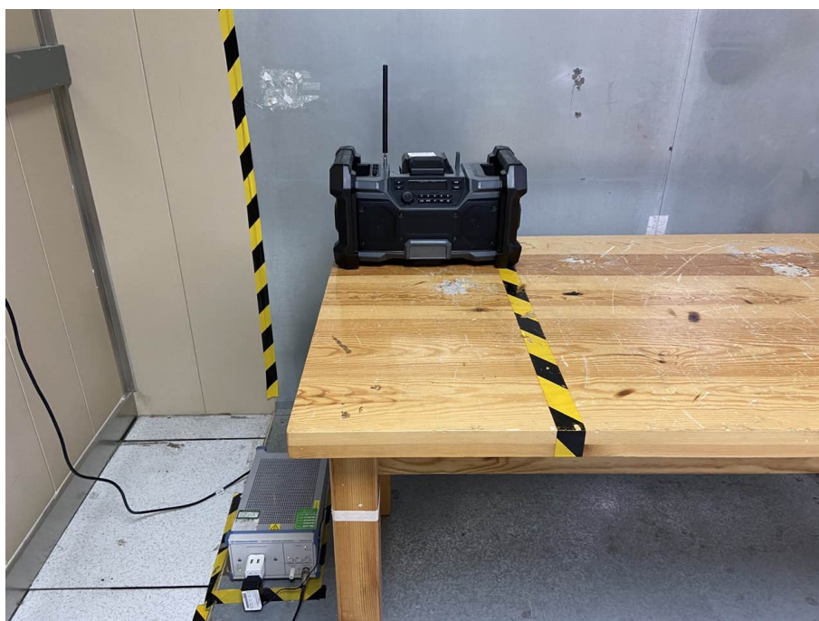
Conducted emission Test Setup
