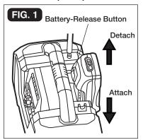
**CAUTION:** Always switch off the unit before removing the battery pack. Align the raised rib on the battery pack with the grooves in the unit, and then slide the battery pack onto the unit.
