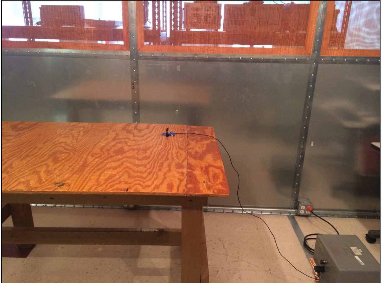
Photograph 3. Conducted Emissions, 15.207(a), Test Setup
