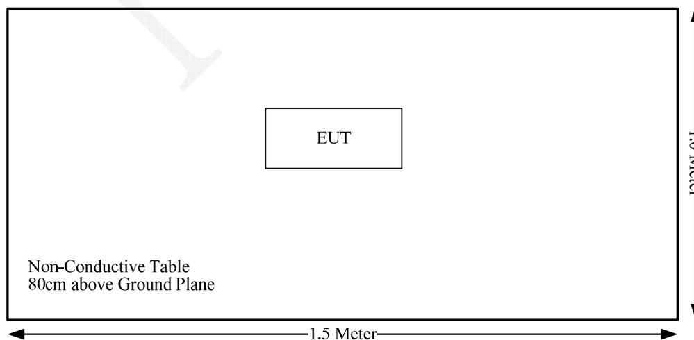
Above 1GHz Radiation Test:
